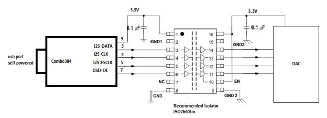
Fig.1 - Isolator between the module and the DAC.
