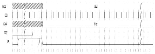
In DSD Mode the I2S\_CLK becomes the DSD clock signal, the I2S\_FSCLK becomes the output data line DSD1 and I2S\_Data becomes the DSD2 Line.
